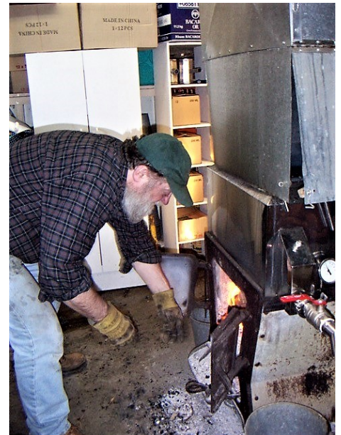
Jay tends the fire under the evaporator where heat transforms sap into syrup.
